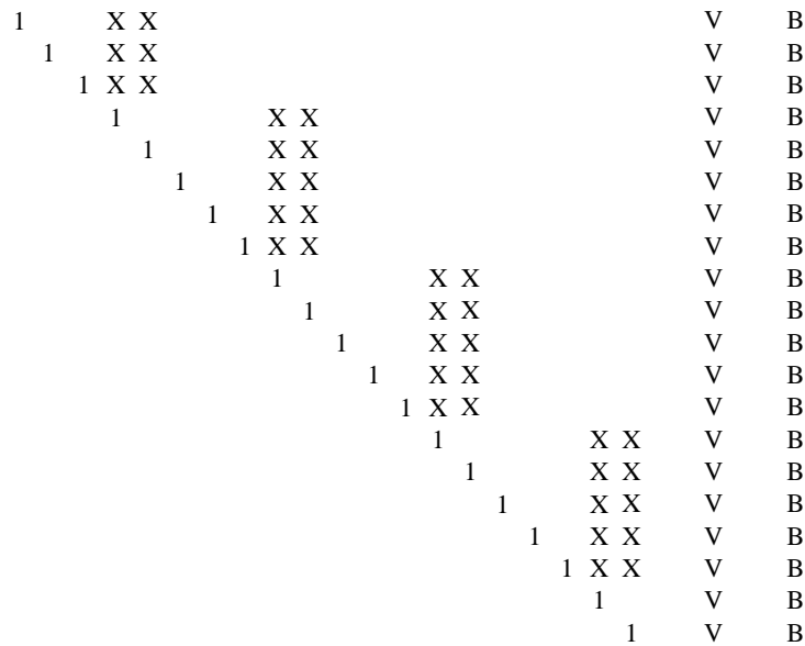
Figure 17.3.2. Target structure of the Gaussian elimination. Once the matrix of Figure 17.3.1 has been reduced to this form, the solution follows quickly by backsubstitution.
